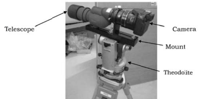
Figure 7 Camera setup from [2]
