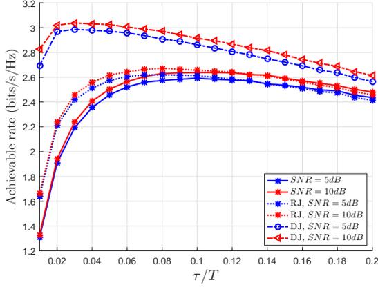
Fig. 2. Average achievable rates of different anti-jamming schemes for  $\varepsilon = 0.1$ ,  $q_t = p_t = q_d = p_d = SNR$ ,  $M = 50$ . The solid curves, dotted curves (with label “RJ”), and dashed curves (with label “DJ”) denote the achievable rates without pilot retransmission (c.f. Proposition 1), with counter strategy for random jamming (c.f. Alg. 1), and with counter strategy for deterministic jamming (c.f. Alg. 2), respectively.
