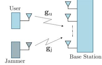
Fig. 1. Massive MIMO uplink with jamming attack.
