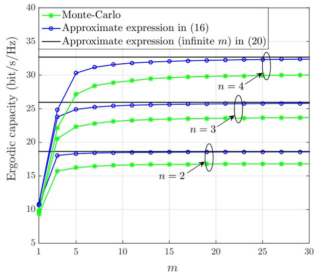
Fig. 3. Comparison of Monte-Carlo simulations with the approximate expressions of the ergodic capacity against  $m$ . Results are shown for  $n = 2, 3, 4$  with  $\alpha = 2.09$ ,  $c_0 = 41.1$  dB,  $\sigma^2 = 5$  dB,  $\sigma_n^2 = -70$  dBm,  $\lambda = 10^{-3} \text{m}^2$ , and  $\rho = 90$  dB.
