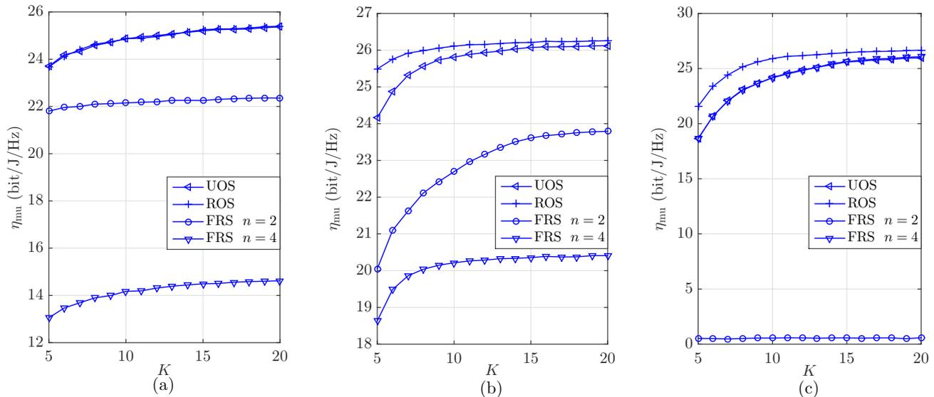
Fig. 9. Energy efficiency for UOS, ROS and FRS versus  $K$  for low/medium/high QoS requirements with fixed  $\lambda$ . (a)  $r_{\text{th}}^k = 10$  bit/s/Hz. (b)  $r_{\text{th}}^k = 20$  bit/s/Hz. (c)  $r_{\text{th}}^k = 30$  bit/s/Hz. Results are shown for  $P_r = 0.25$  W,  $\alpha = 2.09$  and  $\lambda = 10^{-3}$  m<sup>2</sup>.
