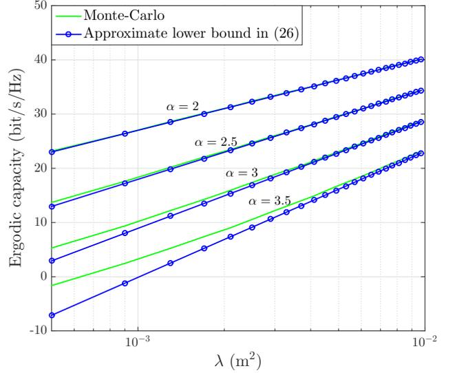
Fig. 6. Comparison of Monte-Carlo simulations and the approximate lower bound of the ergodic capacity in (26) against  $\lambda$ . The results are shown for  $4 \times 4$ ,  $c_0 = 41.1$  dB,  $\sigma^2 = 5$  dB,  $\sigma_n^2 = -70$  dBm, and  $\rho = 90$  dB.
