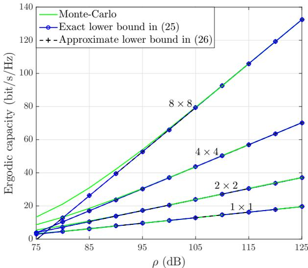
Fig. 5. Comparison of Monte-Carlo simulations, approximate analytical and exact analytical expressions of the ergodic capacity in C-RANs. The different antenna configurations are denoted as  $m \times n$ . Results are shown for  $\alpha = 2.09$ ,  $c_0 = 41.1$  dB,  $\sigma^2 = 5$  dB,  $\sigma_n^2 = -70$  dBm, and  $\lambda = 10^{-3} \text{m}^2$ .
