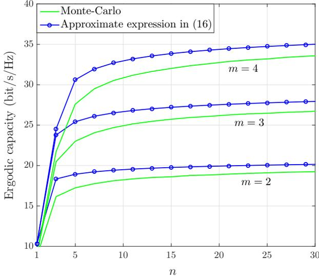
Fig. 4. Comparison of Monte-Carlo simulation with the analytical approximations on the ergodic capacity against  $n$ . Results are shown for  $m = 2, 3, 4$  with  $\alpha = 2.09$ ,  $c_0 = 41.1$  dB,  $\sigma^2 = 5$  dB,  $\sigma_n^2 = -70$  dBm,  $\lambda = 10^{-3} \text{m}^2$ , and  $\rho = 90$  dB.
