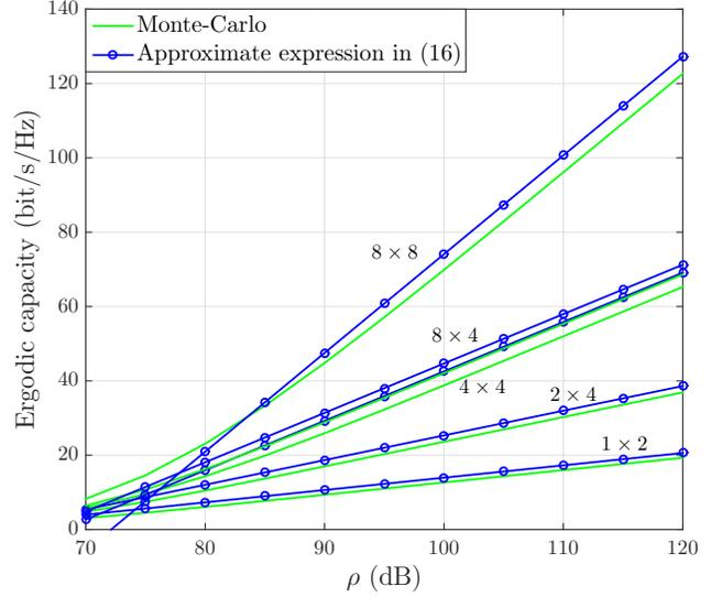
Fig. 2. Comparison of Monte-Carlo simulations with the approximate expressions of the ergodic capacity against  $\rho$ . The different antenna configurations are denoted as  $m \times n$ . Results are shown for  $c_0 = 41.1$  dB,  $\sigma^2 = 5$  dB,  $\alpha = 2.09$ ,  $\sigma_n^2 = -70$  dBm, and  $\lambda = 10^{-3} \text{m}^2$  [30, 34].
