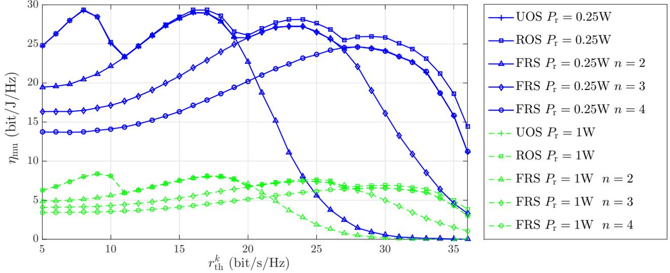
Fig. 7. Energy efficiency for UOS, ROS and FRS versus the different QoS with consideration of both power consumption by signal transmission and reception. We choose  $c_0 = 41.1$  dB,  $\sigma^2 = 5$  dB,  $\lambda_R = 10^{-3}$  m<sup>2</sup> and  $\lambda_u = 10^{-4}$  m<sup>2</sup>.
