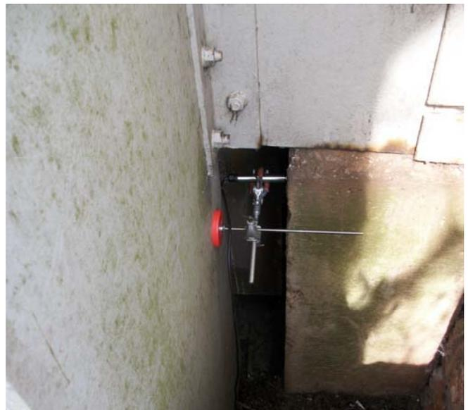
Figure 9, Location and arrangement of LVDT sensor (a) Location, (b) Arrangement
