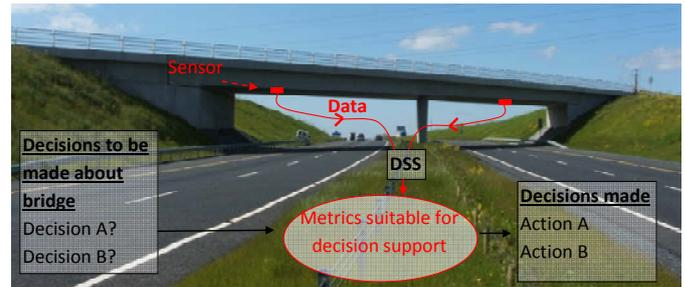
Figure 2. Flow chart showing concept behind DSS.
