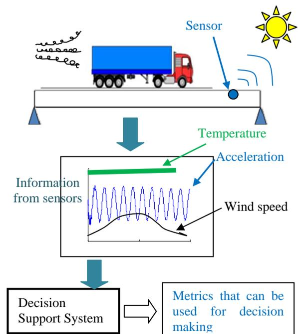
Figure 3. Sequence for using new Decision Support System.
