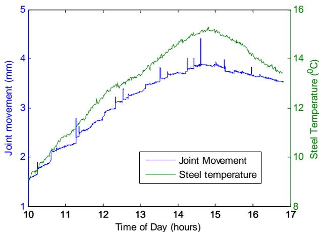
Figure 10, Steel temperature an associated joint movement.
