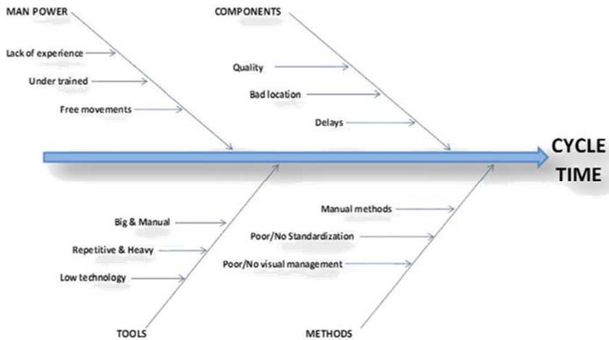
Fig. 4. Assembly process cause-effect diagram.
