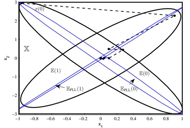
Fig. 1. The constraint set  $\mathbb{X}$ , the PPI sequence  $\{\mathbb{E}(i)\}_{i \in \mathbb{Z}_{[0, 1]}}$  computed applying the method presented (black) and the trajectory of the closed-loop system starting from  $x(0) = [-0.9713 \ 2.9531]^\top$  (dashed black), and the PPI sequence  $\{\mathbb{E}_{\text{PLL}}(i)\}_{i \in \mathbb{Z}_{[0, 1]}}$  computed applying the PLL (blue).
