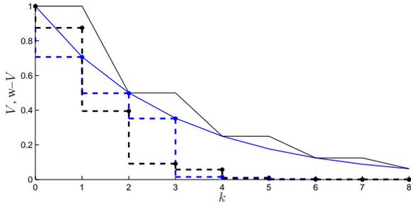
Fig. 2. The Lyapunov functions ( $V$ ) obtained from the synthesis method presented (dashed black) and from application of the PLL (dashed blue), evaluated along the trajectory of the initial condition  $x(0) = [-0.9713 \quad 2.9531]^T$ . The worst-case decrease of the Lyapunov functions ( $w-V$ ) is shown in black and blue line respectively.
