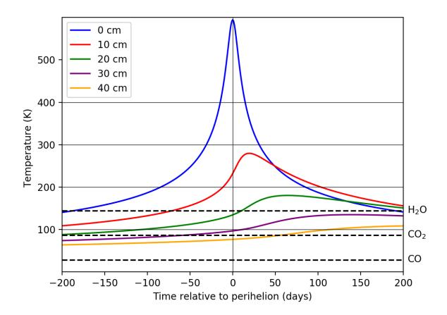
**Figure 4** Thermal modelling of 1I/2017 U1 during its flyby of the Sun, demonstrating the survivability of subsurface ice. Solid lines show the temperature at various depths against time from perihelion in days. Vacuum sublimation temperatures for pure ices are shown as dashed lines<sup>32</sup>. See Methods for details. The spectra of 1I/2017 U1 described in this work were acquired 46 and 48 days after perihelion.
