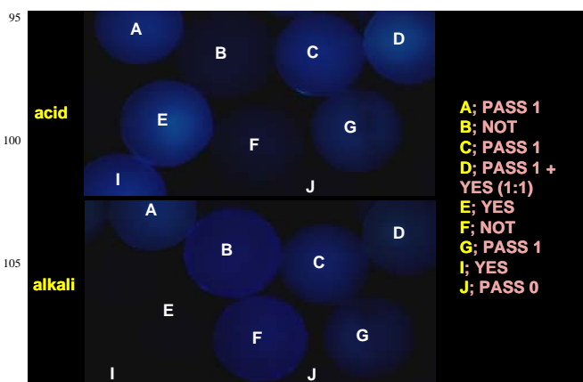
Figure 5. Fluorescence micrographs demonstrating molecular computational identification (MCID) of polymer beads. The beads are tagged with different logic gates and treated with (top) acid and (bottom) alkali in aqueous methanol (1:1, v/v) under ultraviolet (366 nm) irradiation. The logic gate types of some of the beads are discussed in the text. Reprinted from ref. 72.
