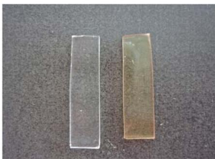
Figure 1. Representative untreated (left) and porphyrin-incorporated (right) hydrogel samples.
