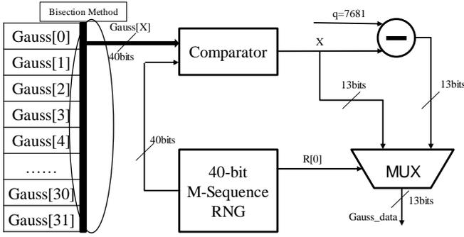
Fig. 1. Hardware structure of the discrete Gaussian sampling.
