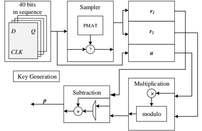
Fig. 3. Hardware architecture of key generation.
