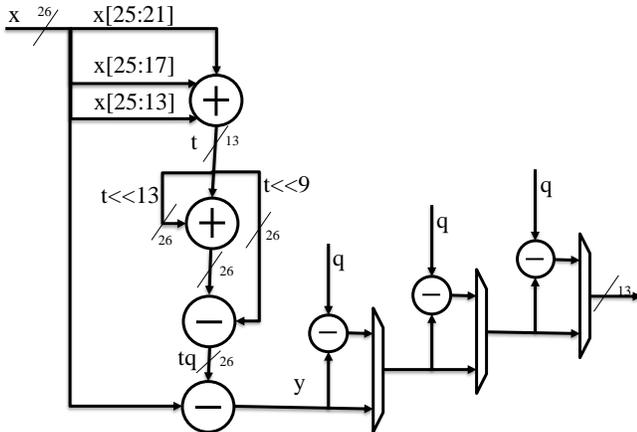
Fig. 2. Hardware structure of the modular reduction.
