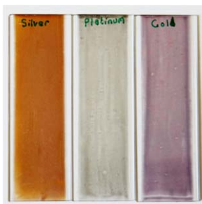
Figure 1: Typical Ag, Pt and Au photodeposited metals on a sol-gel TiO 2 film, created using the standard metal inks, a UVA irradiance of 2 mW cm -2 and irradiation times of, 10 s (for Ag) and 10 min (for Pt and Au).
