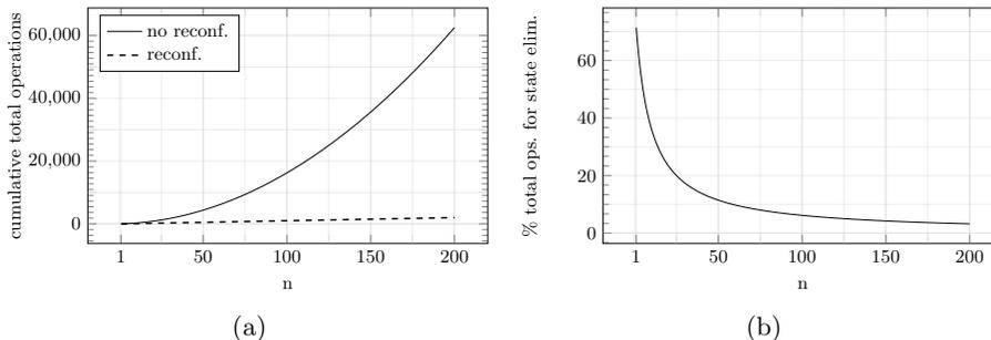
Fig. 4: Cumulative total of arithmetic operations performed for iterative analysis of Zeroconf for  $n = 1 \dots 200$  (a), and the ratio of total operations for reconfiguration to total operations for regular state elimination, given as a percentage (b).
