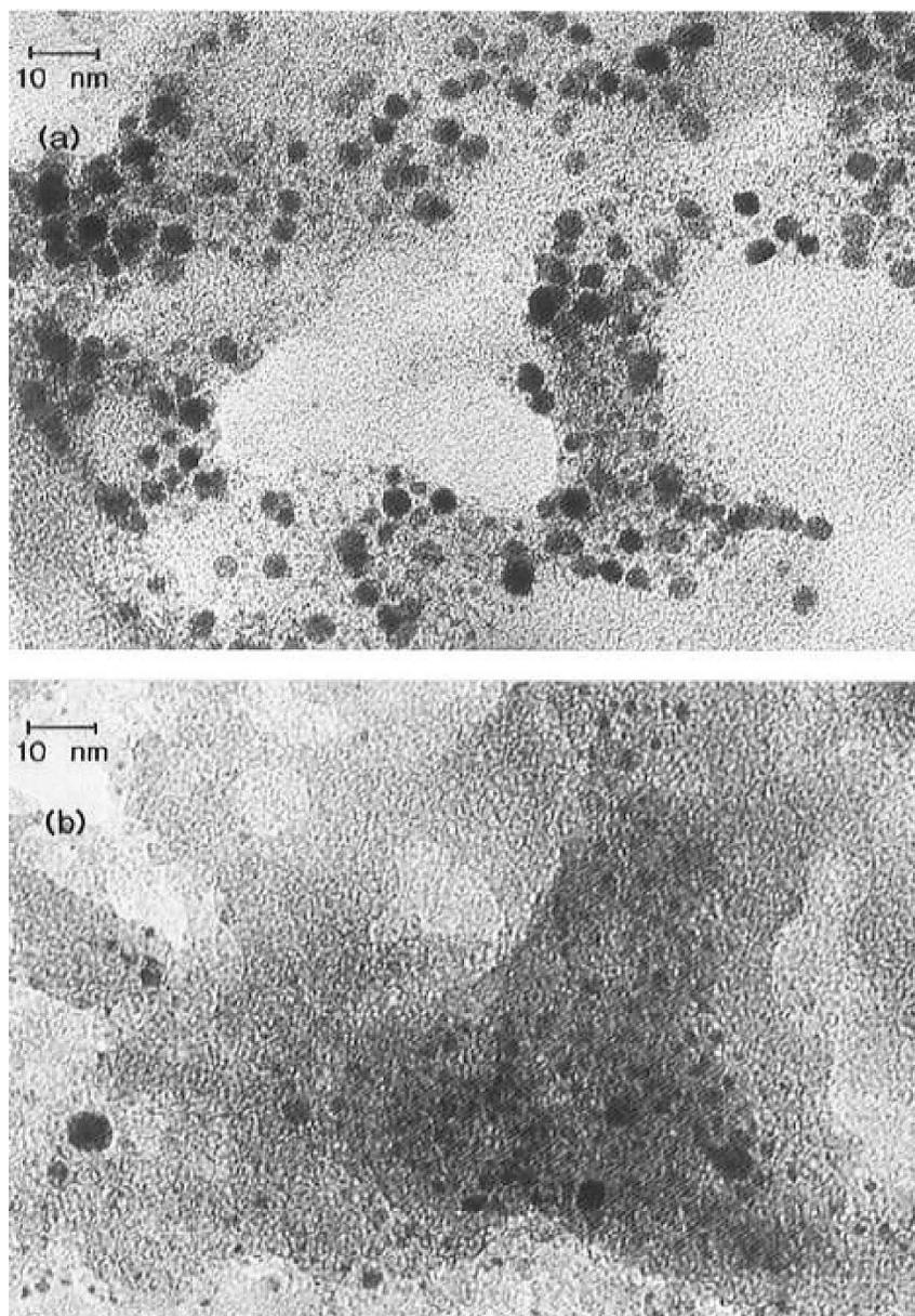
Figure 2:<sup>167</sup> TEM Micrographs of 0.6 wt. % Pt/Al<sub>2</sub>O<sub>3</sub>; sintered (a) and re-dispersed (b)
