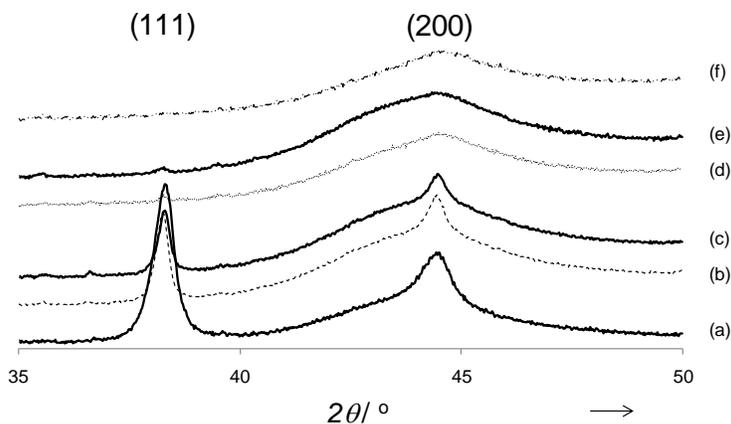
Figure 5:<sup>188</sup> X-ray diffractograms of Au/C catalysts. As received (a), and after treatment with iodomethane for 1 (b), 5 (c), 15 (d), 30 (e) and 60 minutes (f)
