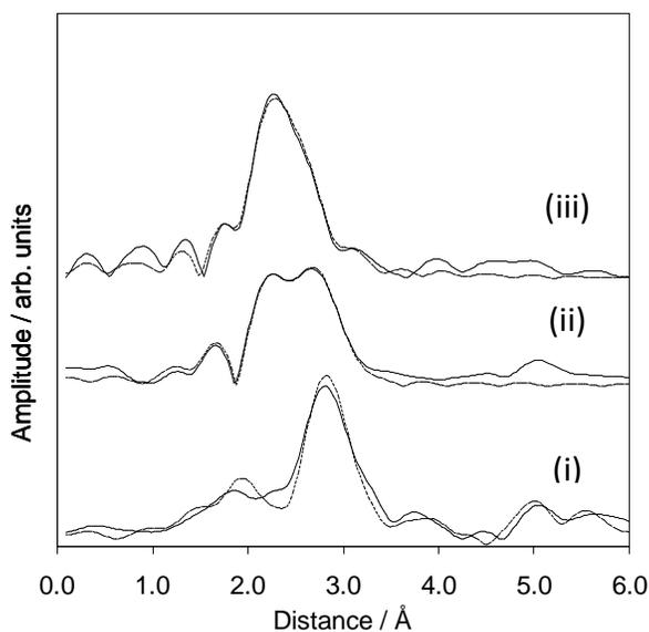
Figure 3:<sup>189</sup> Comparison of experimental (solid) and fitted (dashed) EXAFS data of Au/C catalyst; as received (i) and after 10 h (ii) and 80 h (iii) of methanol carbonylation reaction
