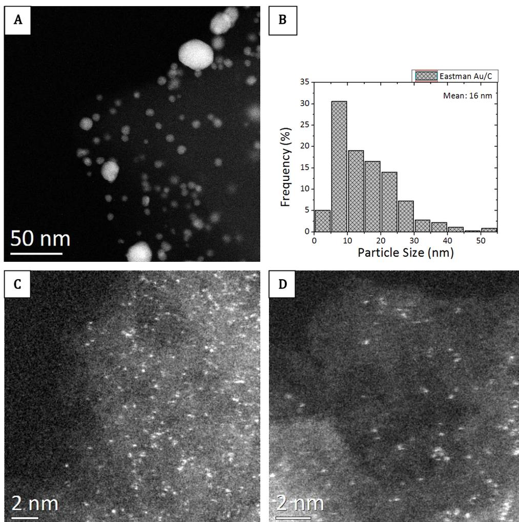
Figure 4:<sup>188</sup> The influence of iodomethane on Au nanoparticles of Au/C. HAADF-STEM images of as received sample (a) and after iodomethane treatment at 240 °C for 1 h (c and d), as well as the particle size distribution of the as received sample (b).
