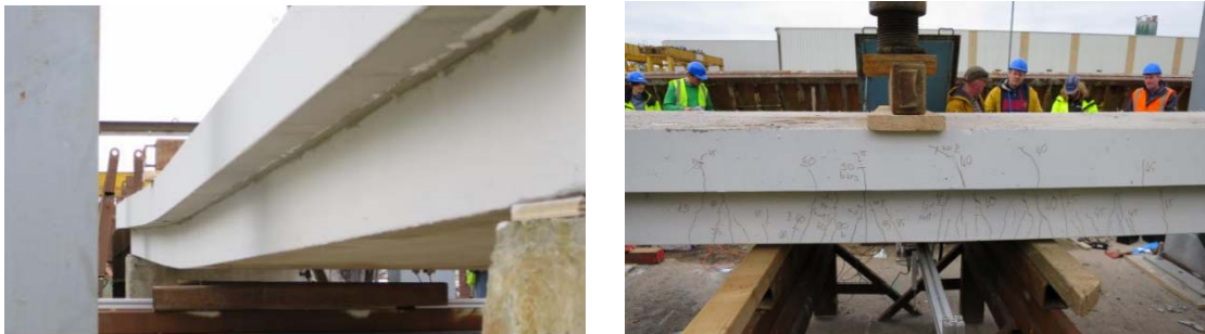
Figure 7 Test beam subject to large deflection and marked crack pattern
