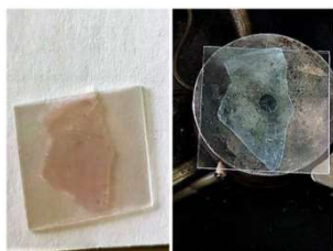
Figure 6. View of PMMA-Co-IL composite film showing colour change from pink (left) to blue (right) after warming on a heating block.
