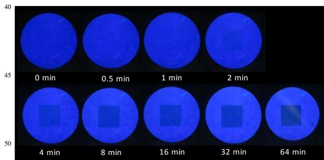
Photographs of fluorescent images after multiple exposure to writing light through the 'square' mask onto the substrate, containing the logical molecular solution including **7** prepared under optimum conditions, for varying cumulative times as noted in each photograph.
