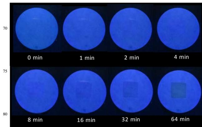
Photographs of fluorescent images after multiple exposure to writing light through the 'square' mask onto the substrate, containing the logical molecular solution including **8** prepared under optimum conditions, for varying cumulative times as noted in each photograph.
