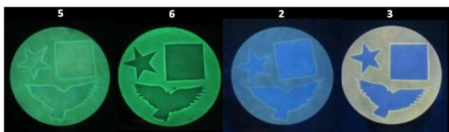
**Figure 7.** Photographs of fluorescent images after single exposure to writing light through a combination of opaque 'square', 'star' and 'bird' masks onto the substrate, containing the logical molecular solution including **5**, **6**, **3** and **2** prepared under optimum conditions, for 35, 16, 35 and 35 min respectively. The square is 4.1 cm side.
