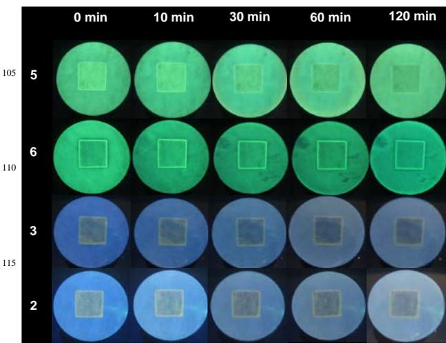
Photographs of fluorescent images after single exposure to writing light through the 'square' mask onto the substrate, containing the logical molecular solution including **5**, **6**, **3** and **2** prepared under optimum conditions, for 35, 16, 35 and 35 min respectively, after standing in the dark for varying cumulative times as noted above each column.
