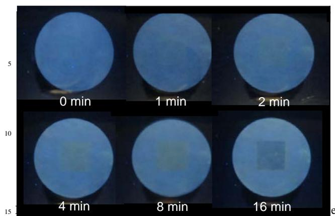
exposure to writing light through the 'square' mask onto the substrate, containing the logical molecular solution including **4** prepared under optimum conditions, for varying cumulative times as noted in each photograph.
