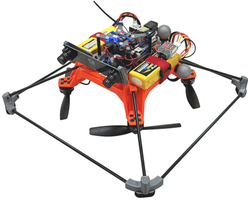
Fig. 4. The inverted quadrotor used in the experiments, which is specifically designed to have a small x/y footprint of 34 cm by 34 cm, a height of 12 cm, and weight of 1.02 kg, to be suitable for indoor flight.
