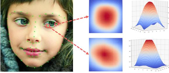
(a) The difference between the heatmap of the eye corner (strong semantic) points and the eye contour (weak semantic) points. Col 2 and 3 represent 2D and 3D heatmaps respectively. In the 3D Gaussian, the  $x, y$  axes are image coordinates and  $z$  axis is the prediction confidence. We can see the 3D heatmap of a weak semantic point has a ‘flat hat’.
