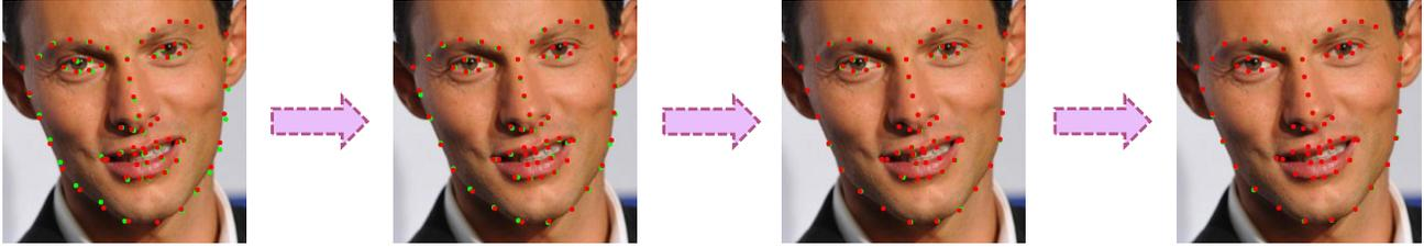
Figure 4. Gradual convergence (one image represents one iteration) from the observation  $\mathbf{o}$  (i.e.  $\hat{\mathbf{y}}$  of the last iteration, green dots) to the estimate of real ground-truth  $\hat{\mathbf{y}}$  (red dots). For last image, the optimization converges because red and green dots are completely overlapped.
