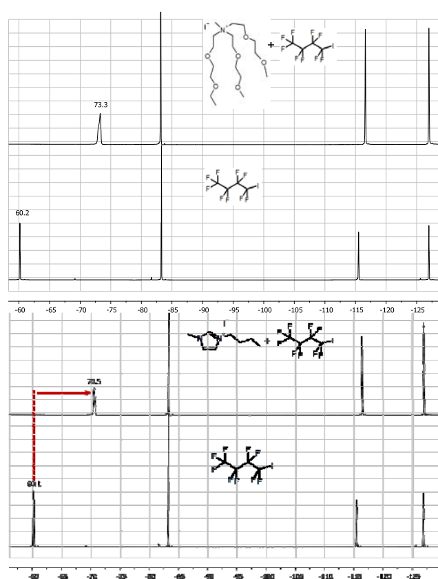
Figure 2: Partial ^{19}F nmr spectra of Top: a mixture of C_4F_9I and [bmim]I; bottom: a mixture of C_4F_9I and ionic liquid, 1 .
