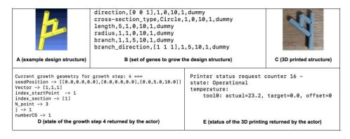
Figure 3. Example of manufacturing a cylinder structure
