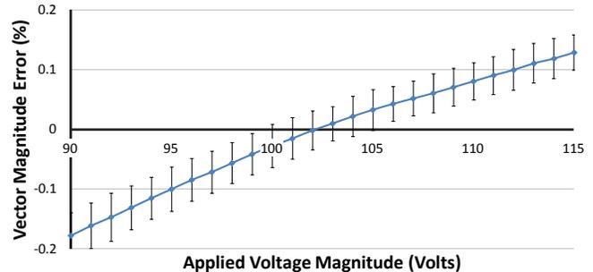
Fig. 4. Amplitude error as percentage of applied voltage.
