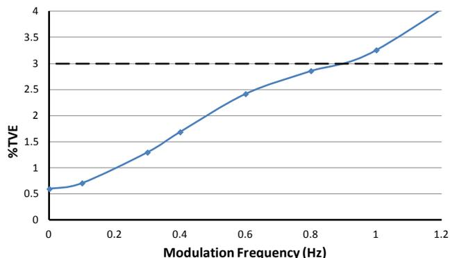
Fig. 6. TVE % versus Modulation Freq. under C37.118.1 subclause 5.5.6.
