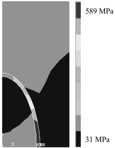
Fig. 3. Stress distribution in the composite for an interface elastic modulus of 1000 GPa and external load of 100 MPa.
