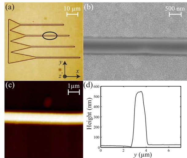
FIG. 1. (Color online) (a) Microscope image of a DLSPW block with four different tapering structures. (b) SEM image of a straight section of a waveguide, revealing a waveguide width of  $w \sim 500$  nm. (c) AFM image of a straight section of a waveguide and (d) cross sectional profile of the AFM image revealing a waveguide height of  $h \sim 550$  nm.
