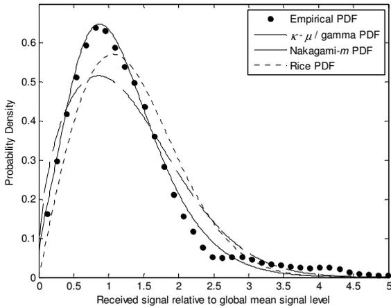
Fig. 4 Empirical PDF and  $\kappa$ - $\mu$  / gamma composite fading PDF for the chest positioned antenna in rotation movement scenario at 5 m during the 1<sup>st</sup> trial. For comparison, Rice and Nakagami- $m$  PDFs are also presented.
