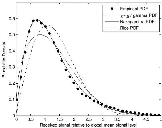
Fig. 5 Empirical PDF and  $\kappa$ - $\mu$  / gamma composite fading PDF for the chest positioned antenna in random movement scenario at 5 m during the 1<sup>st</sup> trial. For comparison, Rice and Nakagami- $m$  PDFs are also presented.
