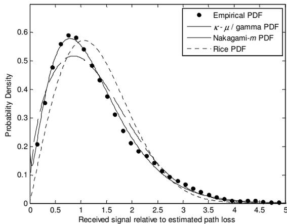
Fig. 3 Empirical PDF and  $\kappa$ - $\mu$  / gamma composite fading PDF for the waist positioned antenna in NLOS walking scenario during the 2<sup>nd</sup> trial. For comparison, Rice and Nakagami- $m$  PDFs are also presented.
