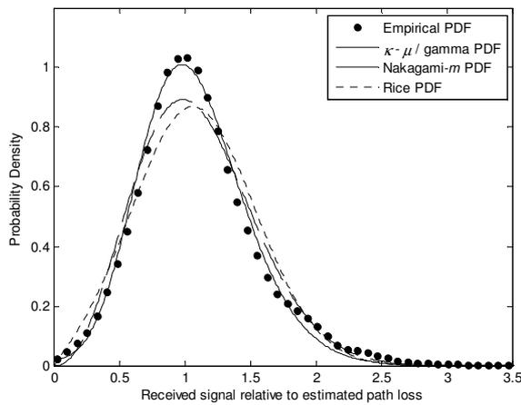
Fig. 2 Empirical PDF and  $\kappa$ - $\mu$  / gamma composite fading PDF for the waist positioned antenna in LOS walking scenario during the 2<sup>nd</sup> trial. For comparison, Rice and Nakagami- $m$  PDFs are also presented.
