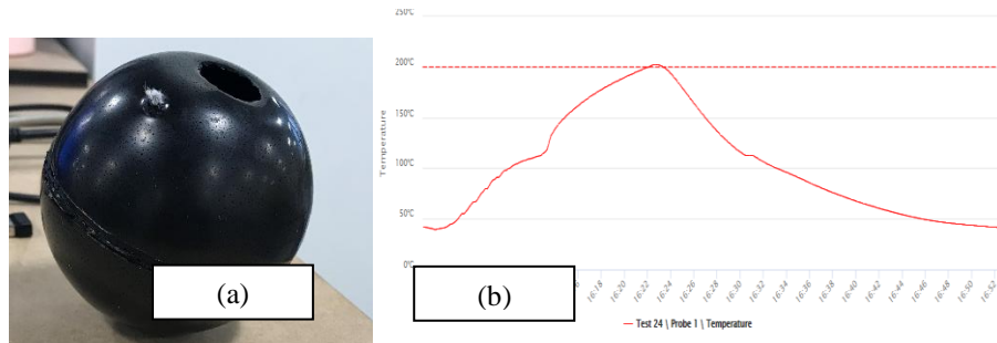
Figure 5 (a)Rotationally Moulded Polyethylene Sphere Sample (b)Sample Internal Air Temperature Trace
