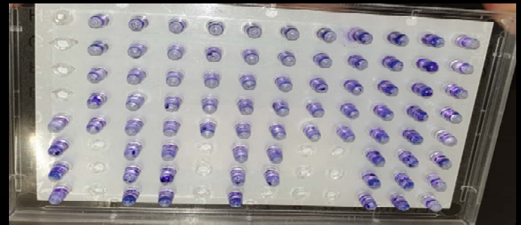
Fig. 3. Shows the CV stained pegs of the MBEC device used for the \phi NFS. As can be seen from left to right an increase in staining and hence biomass as the phage titre decreases in value resulting in less biofilm degradation
