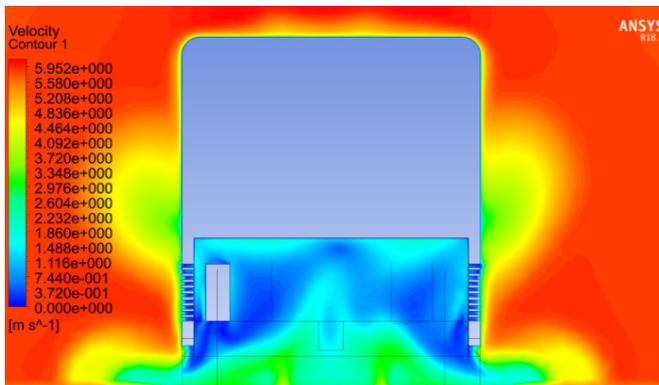
**Fig. 2** Air velocity contours at the engine bay
