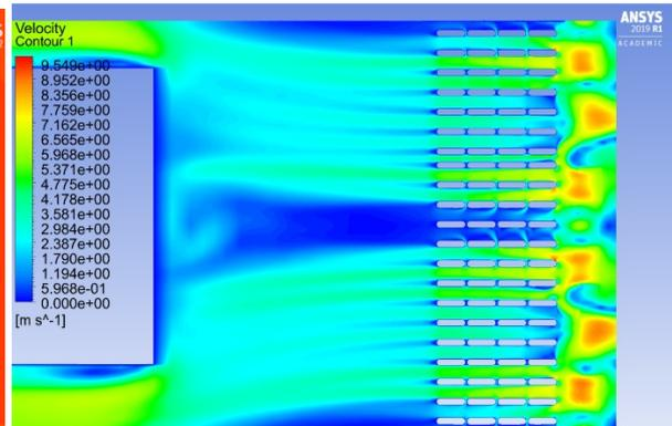
**Fig. 3** Air velocity contours between the tubes
