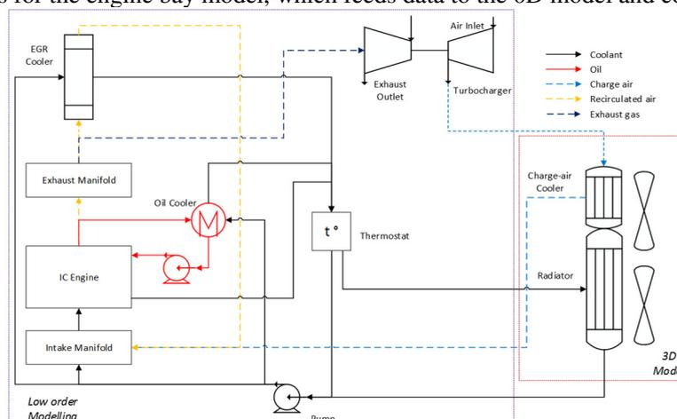
Fig. 1 Schematic diagram of the integrated model
