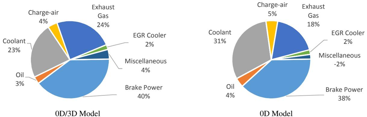
**Fig. 4** Thermal Energy Balance
