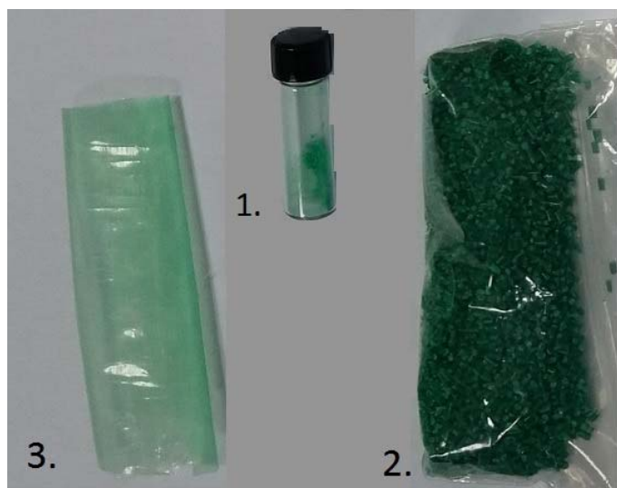
Fig. 1. Images of the PS-DVB based sensor powder pigment (1), extruded LDPE sensor pellet masterbatch (2) and final extruded O 2 -sensitive polymer film (3).
