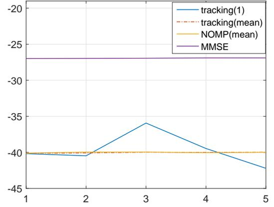
Fig. 2: MSE performance of the NOMP and the tracking algorithms. The tracking algorithm can reach comparable performance as NOMP algorithm with much fewer pilots.
