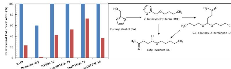
**Figure 1.** Comparison of various catalysts for alcoholysis of furfuryl alcohol to butyl levulinate. Reaction conditions: FA:butanol 1:20, catalyst wt. 0.3 g, temperature 110 °C, (■) Conversion of FA, (■) Yield of BL.
