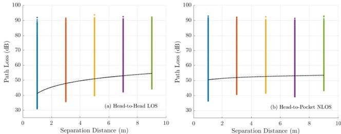
Fig. 2. Scattered measured data along with the path loss fit for the (a) head-to-head (H2H) LOS and (b) head-to-pocket (H2P) NLOS.
