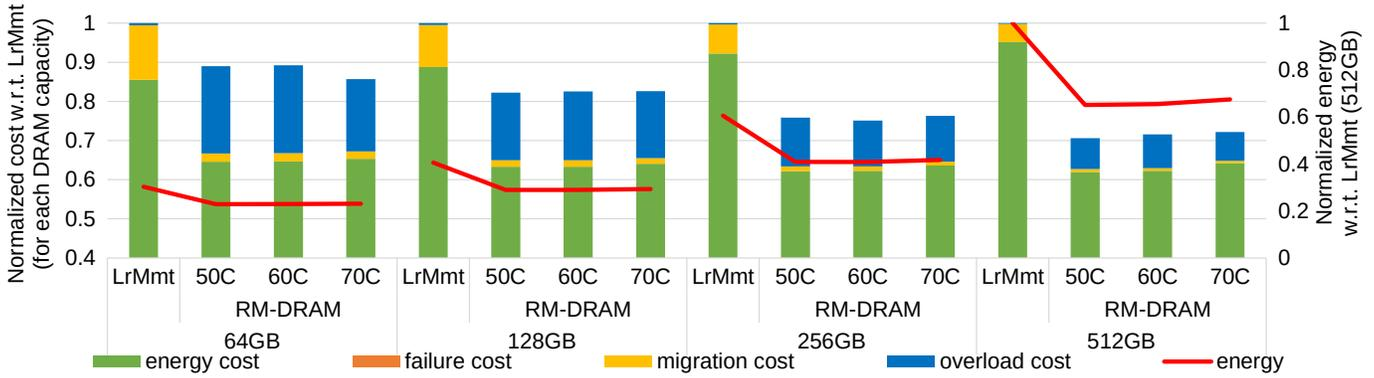
Fig. 5: Relative cost (left y-axis, bars, normalized w.r.t. *LrMmt* at the same memory capacity) and relative energy consumption (right y-axis, lines, normalized w.r.t. *LrMmt* at 512GB), for the same target node utilization. Left y-axis starts at 0.4.
