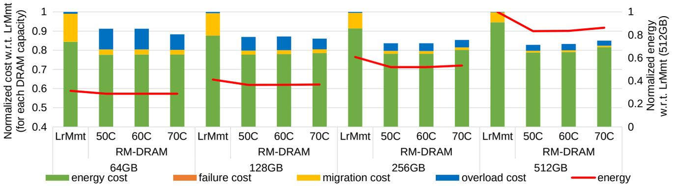
Fig. 4: Relative cost (left y-axis, bars, normalized w.r.t. *LrMmt* at the same memory capacity) and relative energy consumption (right y-axis, lines, normalized w.r.t. *LrMmt* at 512GB), for effectively equal node utilization. Left y-axis starts at 0.4.
