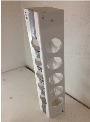
Figure 2.18. A simple collector prepared at QUB from 65mm drainpipe with holes for water flow. A lateral cut has been made and resealed to allow later removal from longlines during deployment.
