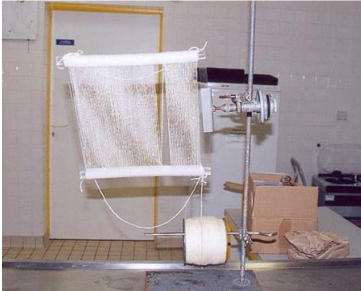
Figure 2.20. CEVA device used to twist the culture string round the collector frame.
