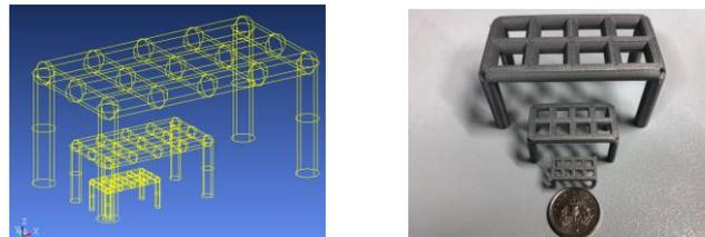
(a) CAD models with different scales (4:2:1) (b) 3D printed structures (4:2:1)
