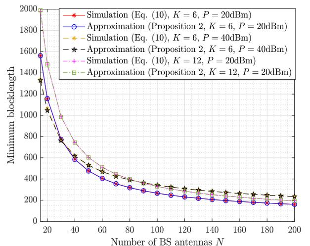
Fig. 5: The minimum blocklength versus the number of BS antennas with  $\eta_k = 0.8$ .
