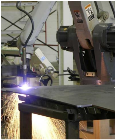
(a) Plasma cutting performed by an industrial robot (Wikipedia 2018a).
