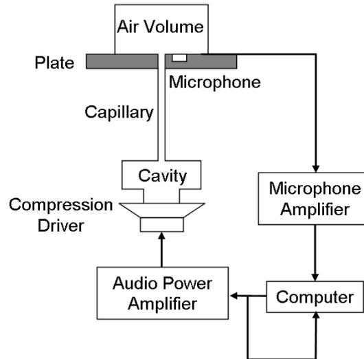
Figure 2 Modified single microphone capillary-based impedance measurement set-up
