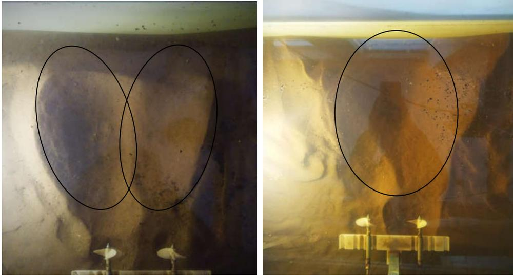
**Figure 4.** ICRTP and ECRTP wall scour structures.
