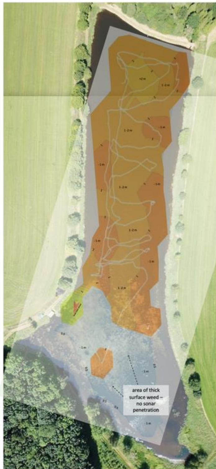
Figure 5. Site 3, where few subaqueous targets occur and weed growth limited sonar deployment by drone or boat due to surface reflections. Flight lines are left on the map, for illustrative purposes.
