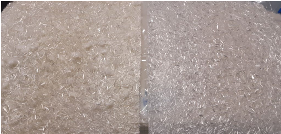
Fig. 1 – Poor (left) and optimum (right) fibre adherence and distribution of a rotationally moulded part.
