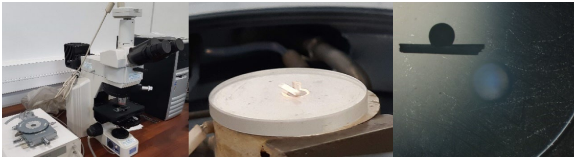
Fig. 2 – Illustration of the setup used for FPIT. Microscope (left), fibre-particle contact (centre) and a 1X picture of the sample (right).
