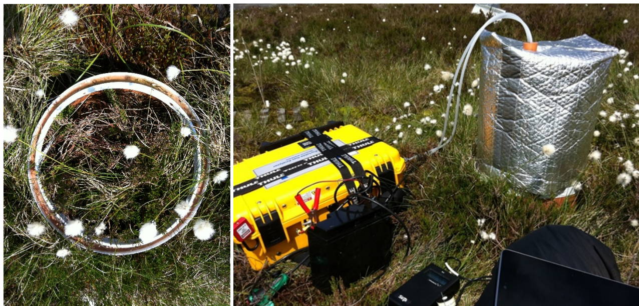
Figure 1. An example collar (left), and demonstration (right) of the use of the on-line Los Gatos Research Ultra-portable GHG Analyzer (UGHGA; Model 915-0011; Los Gatos Research, Mountain View, California) for CH 4 flux measurement using a shrouded chamber.
