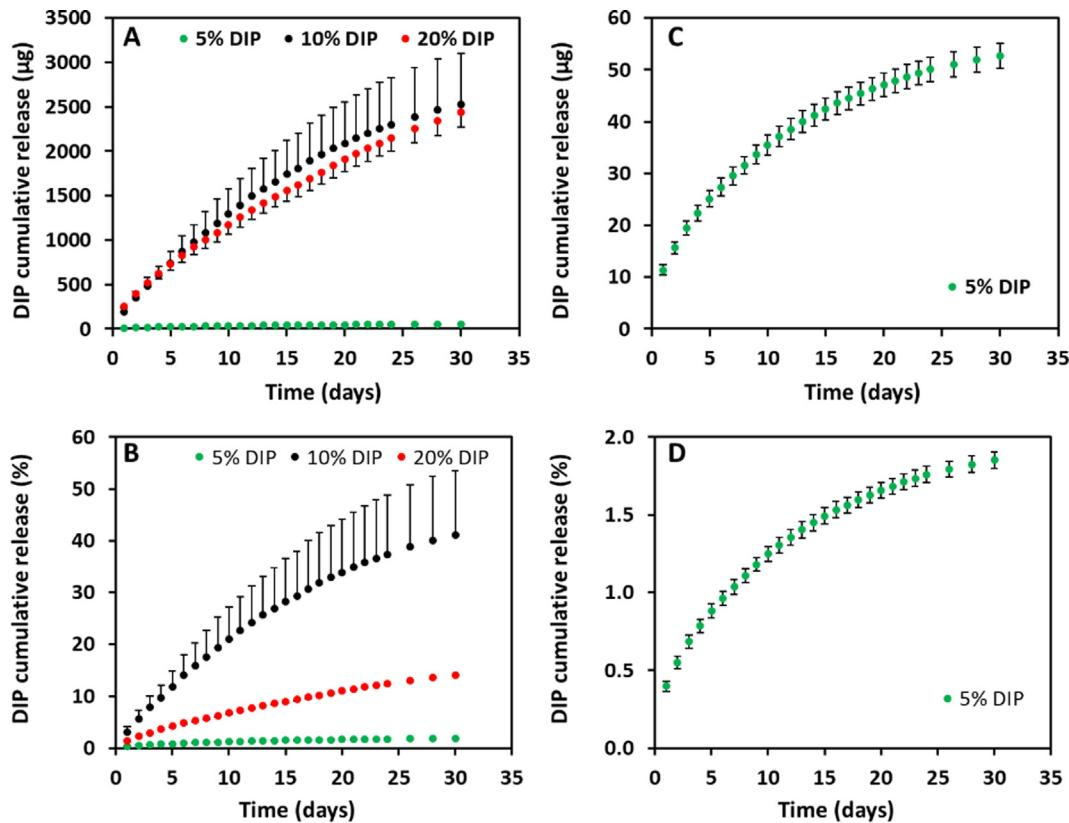
**Fig. 8.** *In vitro* DIP release curves from DIP-loaded 3D-printed samples up to 30 days in PBS at 37 °C expressed in µg as function of time (A) and expressed in percentage as a function of initial DIP drug loading (B) ( $n = 4$ ). Figures C and D represent curves of the 5% DIP-loaded 3D-printed samples in a different scale expressed in µg as function of time, and expressed in percentage as a function of initial DIP drug loading, respectively.
