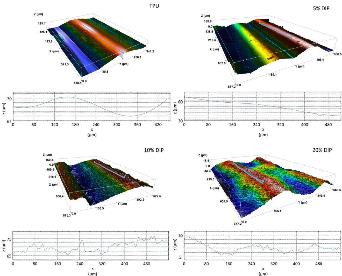
**Fig. 5.** 3D images of the tubular grafts' surfaces containing different DIP concentrations and their topographic profiles studied in the direction of the predominant surface pattern determined by the 3D printing methodology.
