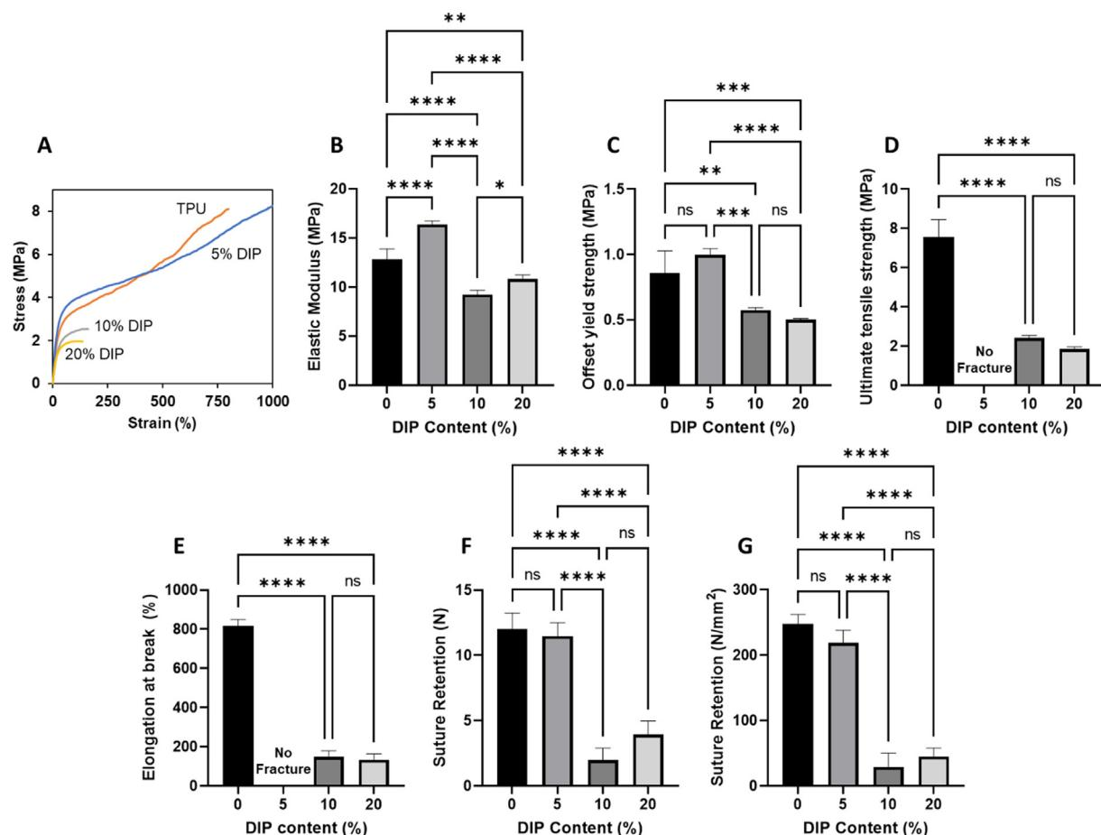
**Fig. 7.** Representative stress/strain curves for the DIP-loaded 3D-printed samples (A). Elastic modulus (B), offset yield strength (C), ultimate tensile strength (D), elongation at break (E) and suture retention strength (F and G) for the DIP-loaded 3D-printed samples ( $n = 4$ ).
