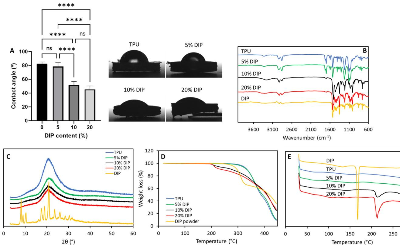
**Fig. 6.** Influence of the DIP content on the contact angle of water with the DIP-loaded 3D-printed samples ( $n = 4$ ). ATR-FTIR spectra (B), XRD diffractograms (C) and TGA (D) and DSC curves (E) of each of the DIP-loaded 3D-printed samples.
