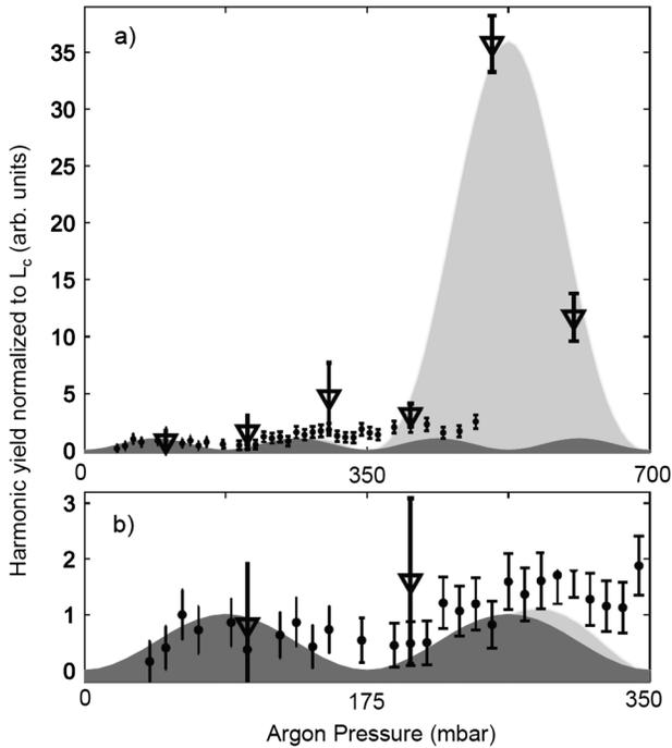
FIG. 4. (a) Comparison of the angularly and spectrally integrated harmonic yield for the 27th harmonic using a 700  $\mu\text{m}$  merged argon jet (circles) and a dual-gas six-sources jet (triangles) which has five hydrogen jets placed between the six argon jets. For comparison the theoretical curves are included for  $N_{\text{QPM}} = 1$  (dark shaded) and  $N_{\text{QPM}} = 6$  (light shaded). (b) Close-up of the merged-jet oscillations with increasing argon backing pressure.
