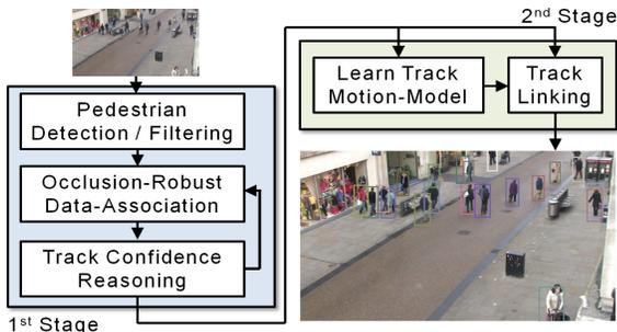
Figure 1. Flowchart of our tracking system.
