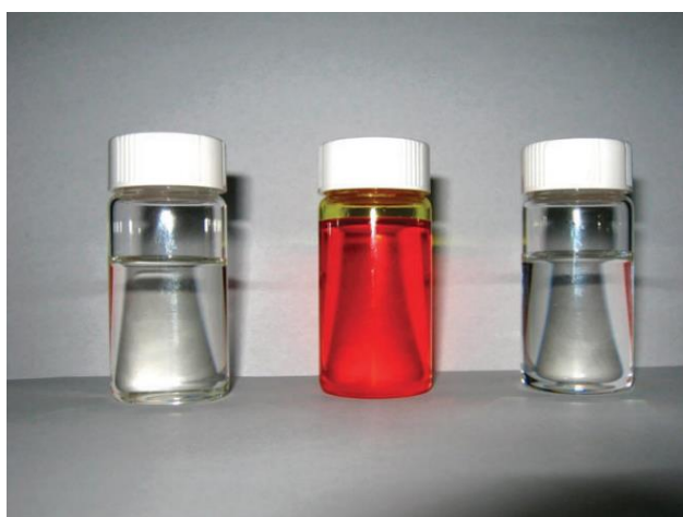
Figure 1-11: the colour change following the addition of 1-methylnaphthalene (right) to liquid 1-ethyl-4-cyanopyridinium bis{(trifluoromethyl)sulfonyl}imide to form liquid charge-transfer complex (centre) at 293K. 12
