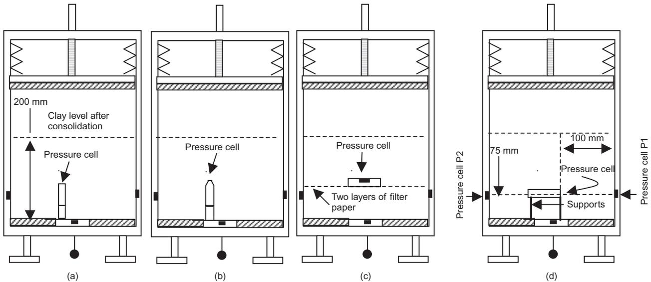
Fig. 4. Probe positions in the testing chamber
