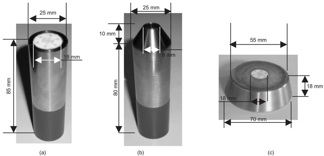
Fig. 1. Miniaturised probe configurations: (a) configuration 1; (b) configuration 2; (c) configuration 3
