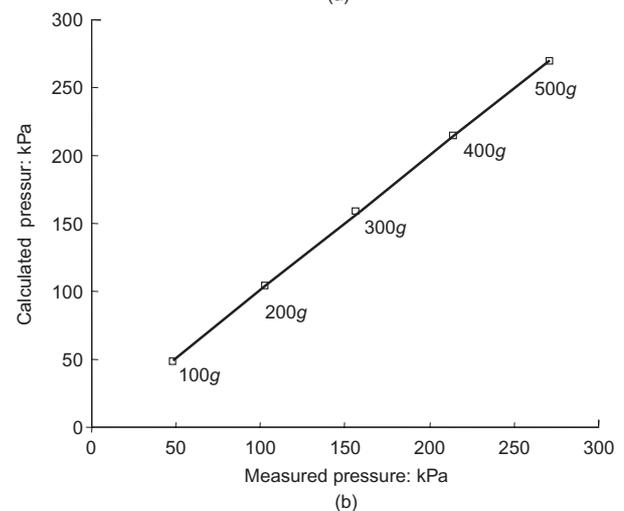
Fig. 11. Probe performance under elevated acceleration
