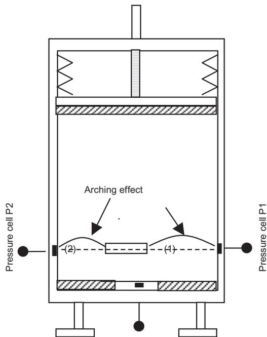
Fig. 10. Probe position and arching effect during Test 5
