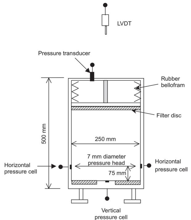
Fig. 3. Testing chamber
