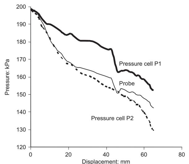
Fig. 9. Probe pressure and external pressure cell readings with vertical displacement
