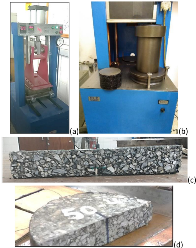
Fig. 1. Sample preparation setup (a) roller compactor (b) gyratory compactor (c) SENB (d) SCB.
