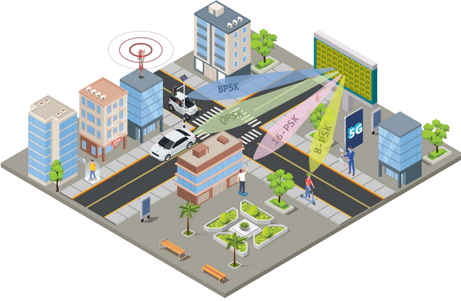
Fig. 1. Illustration of a RIS as an access point within a cell-free network of a smart city. The RIS, mounted on a billboard, modulates and steers beams tailored to individual users.
