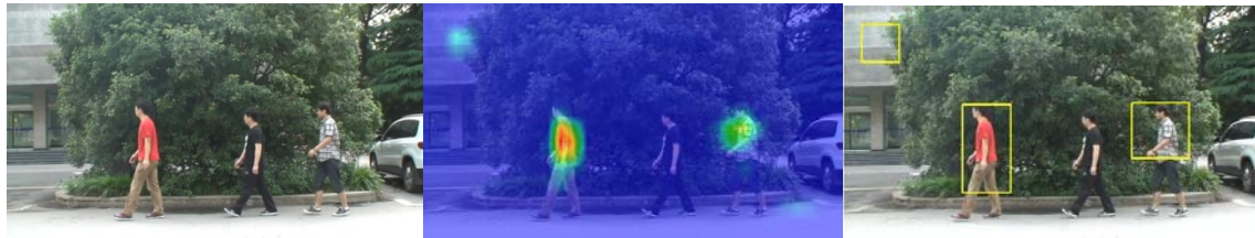
(a) 视频帧 (b) Itti 显著图 (c) 行人检测结果 (a) video frame (b) Itti saliency map (c) People detection
