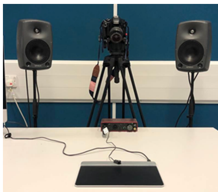
Figure 1. The prototype instrument used in the research study consisted of a 2D pressure sensor and contact mic, both connected to a Macintosh computer (out of shot) running the synthesis software, which outputted audio through two floor mounted speakers. The video camera was used to record gesture data during the study. Reproduced with permission from Smith et al. (2023).
